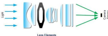
Optical aberrations occur when points in the image do not translate back onto single points after passing through the lens — causing image blurring, reduced contrast or misalignment of colours (chromatic aberration). Lenses may also suffer from uneven, radially decreasing image brightness (vignetting) or distortion. Now I don't know about you, but that's all a bit technical, so I won't delve any further into it.
